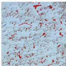
Figure 1: Silicon filter with atmospheric deposition of microplastics. Particles were selected in the size range of 25 \mu\text{m} – 1.5 mm.
