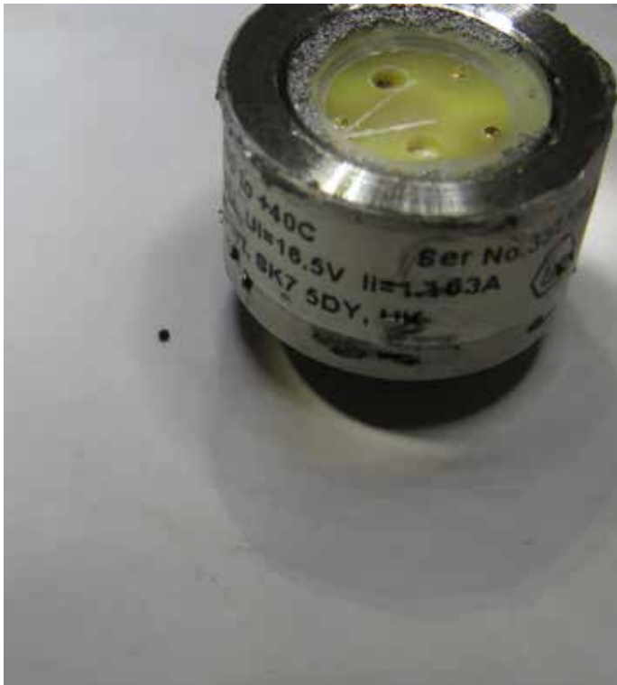
Left: the sensor bead in the housing, right: sensor bead compared to the housing, with a diameter the size of a 10c piece.
