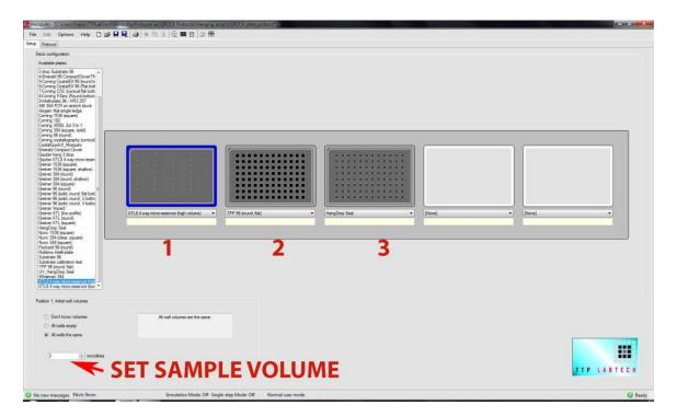
LCP Mosquito Set-up tab: The protein (sample) strip goes in position 2.
