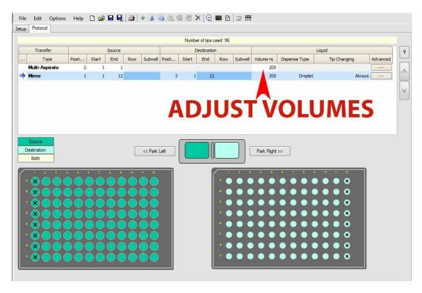
**On the Set-Up tab** make sure all positions are correctly assigned. Again you should not have to change anything here except for the volume of sample if you have 2 uL of sample use XLT8 (low volume) and if you have 5 uL of sample use XLT8 (high volume).
