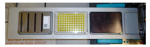
The LCP Mosquito deck is shown below: the condition plate is on the left; the protein sample/s is placed in plastic strips in the holder in the middle; and the hanging drop seal is placed on the holder (substrate) on the right.
