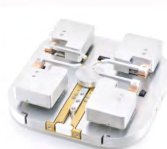
In situ nano-manipulation, electrical and mechanical testing
